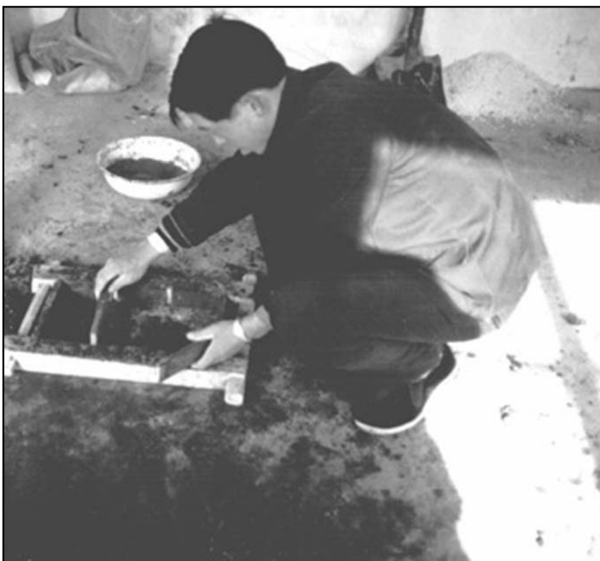
Figure 1 Adjusting rammed-earth brick mould for use with UMB in North China (Gansu Province).
