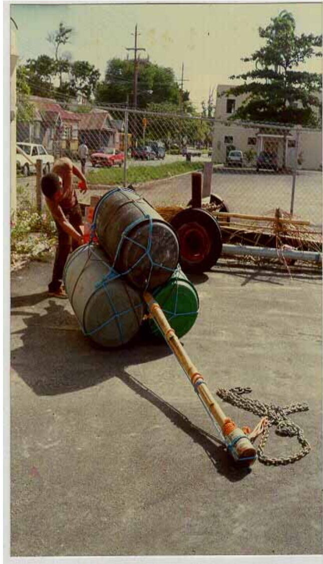
Figure 3: Bottom end of surface section of experimental FAD.
