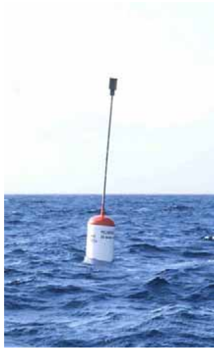
MKII-GRP7 Medium strength current 560 m mooring depth
