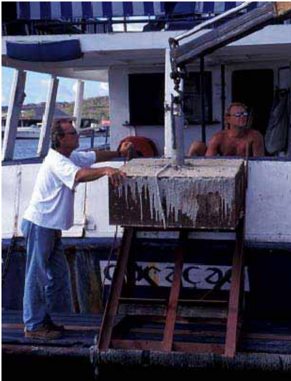
Old type anchor (1 260 kg) Being lowered on ramp
