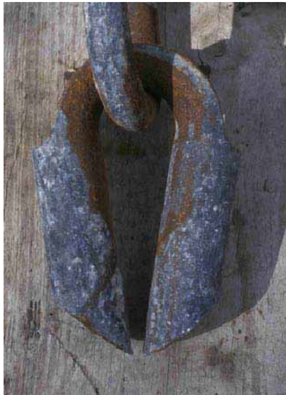
Galvanized connector, of inferior quality
