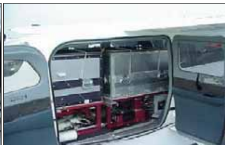
FIGURE 7.5 Release system installed inside a Cessna 206 aircraft.
