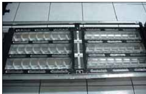
FIGURE 7.4 Screw auger system for chilled adult release.
