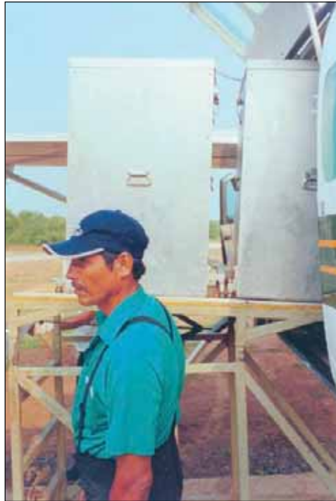
FIGURE 7.3 Release machine with a capacity of 10 million sterile flies per load.
