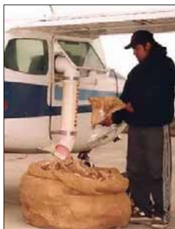
FIGURE 7.1 Typical chute used in aircraft for paper bag aerial release.
