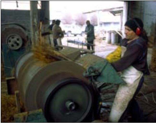
Larger-scale producers use electric machines to strip the bark
