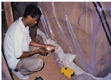
FIGURE 19 Measuring phosphine gas concentration in stack covered with thick polythene sheeting and anchored to ground with sand snakes
