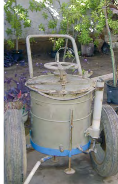
Figure 2. A large movable fertilizer applicator with a manual mixture.
