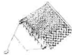
Dredge with teeth, on the lower edge of the frame and with depressor flap on the upper edge Weight 70-100 kg
