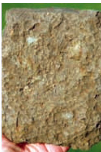
MODERATE CONDITION VS = 1 Soil has common (10–25%) fine and medium orange and grey mottles.
