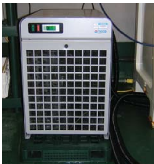
Figure 5.10: A combined heater/chiller unit suitable for use in conjunction with a small-scale standard design system
