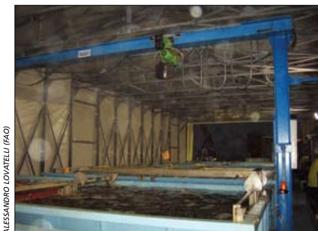
Figure 8.1: Mechanical system for loading and unloading tanks
