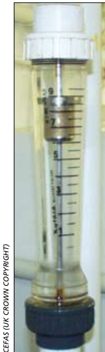
Figure 5.9: In-line flow meter used in a depuration system
