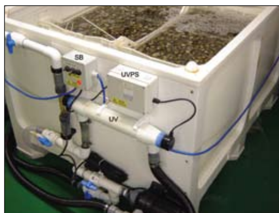
Figure 6.3: UV unit attached to a small-scale shallow tank system
