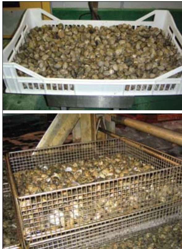
Figure 5.6: Example of trays suitable for use in a depuration tank
