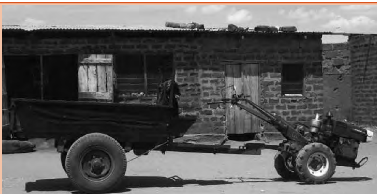
FIGURE 19 Single axle tractor and trailer (Photo by J. Kienzle)
