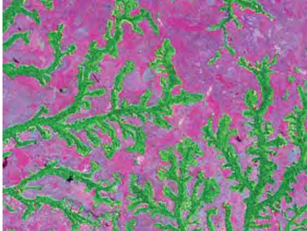
FIGURE 2.30 Band and enhancement combinations that highlight the gallery forests that are typical for parts of Central and West Africa
