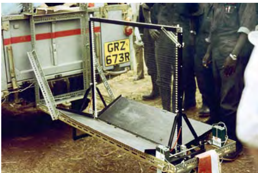
FIGURE 3.4 Vehicle-mounted electric screen for monitoring Glossina morsitans
