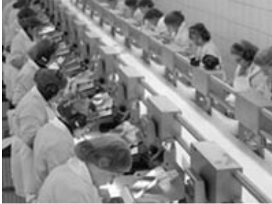
FIGURE 1 A typical fish processing flowline may employ up to 20-30 operators, carrying out trimming that is checked afterwards by quality inspection
