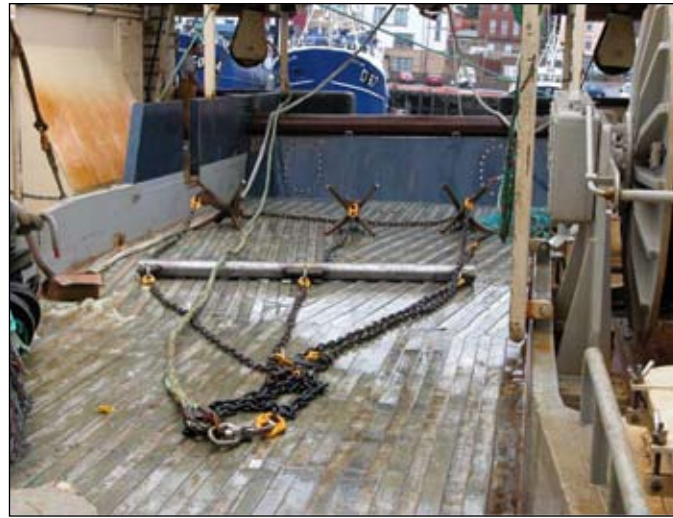
FIGURE 14 Creeper gear for recovery of gillnets on board the MFV India Rose
