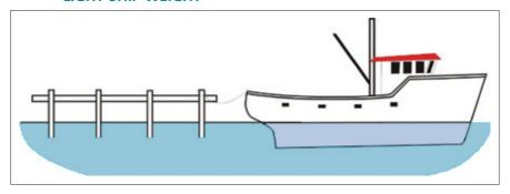
The light ship weight is the actual weight of a vessel when complete and ready for service but empty.
