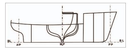
When the shape of the hull of a vessel is known, the designer, often a naval architect, can calculate the centre of buoyancy (B) for the various combinations of displacement, trim and heel.
