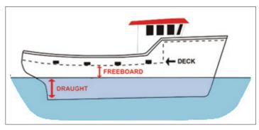
Draught relates to the depth of water required for a vessel to float freely and is measured vertically from the underneath side of the keel to the waterline.
