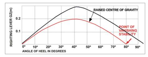
Raising the vessel's centre of gravity (G) causes a decrease in the metacentric height (GM) and thereby smaller values of the righting levers (GZ).
