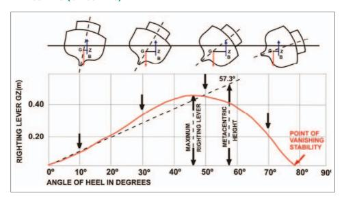
Stability curves (**GZ** curves) are used to show graphically the stability levers (**GZ**) exerted by a vessel to return itself to a position of equilibrium from the various conditions of heel. The curves have several general characteristics and the following factors should be observed:
