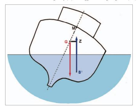
Should the vessel's centre of gravity (G) be near the metacentre (M) the vessel will have only a small metacentric height (GM) and the righting lever (GZ) will also be a small value. Therefore, the moment of statical stability to return the vessel to the upright position will be considerably less than that of the previous illustration.
