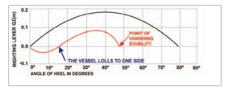
If the vessel's centre of gravity (G) is above the metacentre (M), the vessel is in an unstable equilibrium. The vessel has a negative GM and is not able to float upright. Either the vessel will capsize of or float at an angle from the upright to one side. (See also the section on loll on page 5).
