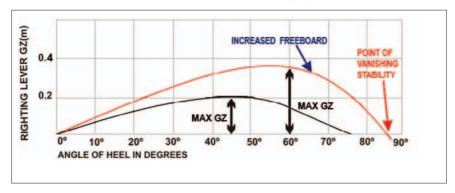
By loading less the vessel will have more freeboard and the values of the righting lever (GZ) will, in general, be higher. The point of vanishing stability will also be higher, i.e. the vessel's ability to return to upright after having been heeled to large angles of heel is better.
