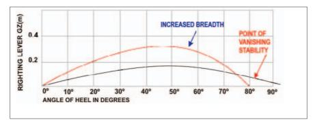
The hull form of a vessel is an important factor in determining the characteristics of its stability. Increased breadth (beam) will result in higher values for metacentric heights (**GM**) and righting levers (**GZ**). However, the point of vanishing stability will be less, i.e. the vessel will capsize at a **smaller** angle of heel.
