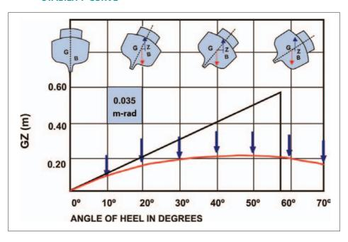
Various methods can be used to calculate the area under the stability curve (GZ). The simplest is to divide the area under the curve into a suitable number of trapezes and calculate their total area (the trapezoidal rule). The area may also be calculated by the so-called "Simson's rules" which is demonstrated below:
