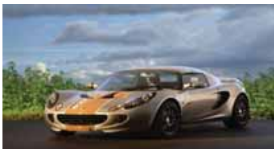
Figure 4. Lotus Eco Elise (launched July 2008) with body panel, spoiler, seats made from natural fibres. Hemp plants growing shown in the background. (with permission)
