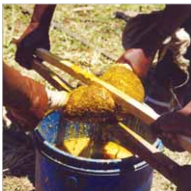
9.10 Using sticks to squeeze the bag of molten beeswax and water Tanzania © NB
