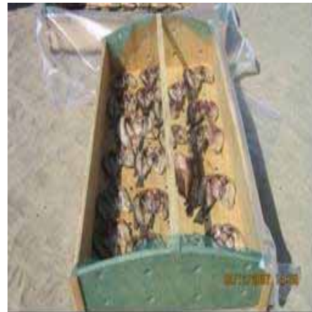
Plate 2. Plywood solar dryer
