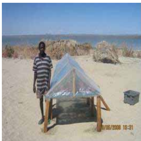
Plate 3. Improved raised fish solar dryer
