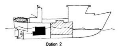
Deckhouse is forward. Access to engine is through a hatch with a high coaming on side. (Engine can be removed through a flush hatch bolted to deck.)
