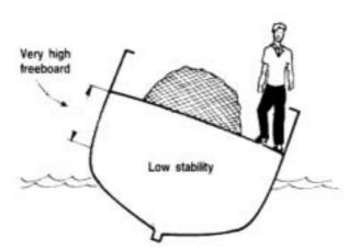
The freeboard is, thus, very important for the safety of a fishing boat. However, if it is increased too much, the boat will lose stability more quickly than a boat with less freeboard. This will happen if heavy fishing gear is put on deck. So, a compromise has to be found to select the optimum freeboard.
