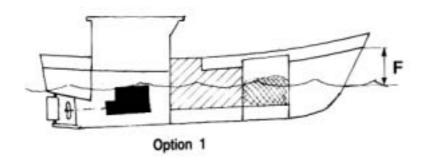
Fish-hold is amidship. Net is in fishing gear-hold during rough weather. Freeboard (F) at the bow should be at least equal to 17 LOA + 700 mm (LOA =10 m, F = 870 mm) for acceptable safety
