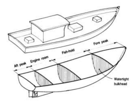
Leaks in the engine room are often caused by a corroded seacock, damaged seawater hoses, poor quality and installation of wet exhaust hose and a faulty stuffing box in the stern tube. If the buoyancy of the aft peak is sufficient, the boat will float.
