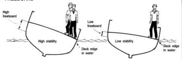
Comparing two boats with the same beam but different freeboards, the one with the higher freeboard has more stability and is able to take more people at the deck edge before the deck touches the water.
