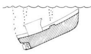
If the boat has no watertight bulkheads and if the bilge pump cannot cope with the leak, the boat will certainly sink.
