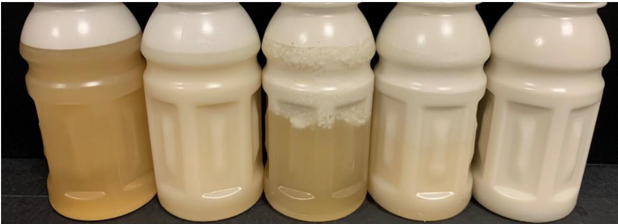
Control OSA 0.4 g/L Gellan 0.05 g/L OSA + Gellan Total: 0.45 g/L (OSA: 0.4, GG: 0.05) OSA 2.4 g/L
