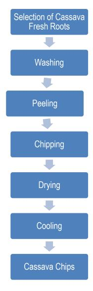
Figure 3: Flowchart for production of Cassava chips
