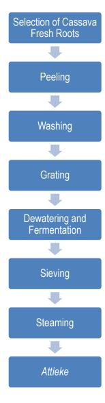
Figure 5: Flowchart for production of Attieke
