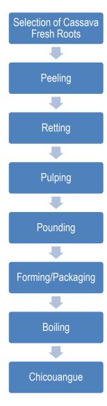
Figure 6: Flowchart for Production of Chicouangue
