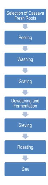
Figure 1: Flow chart for production of gari
