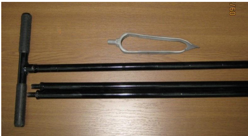
Manual soil drills to take soil samples at different depths
