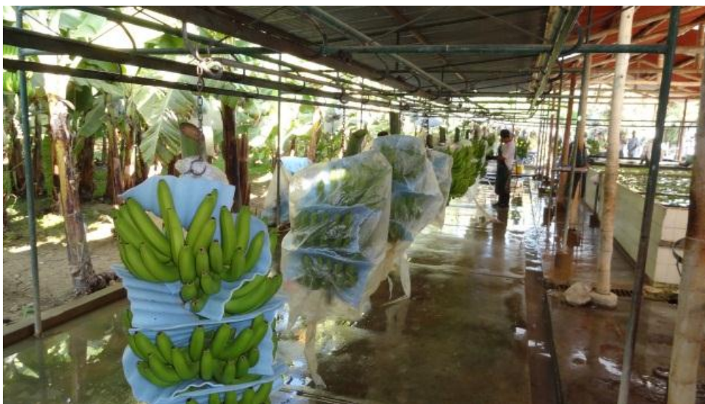
Banana bunches arrive at the packing station via the cableway
