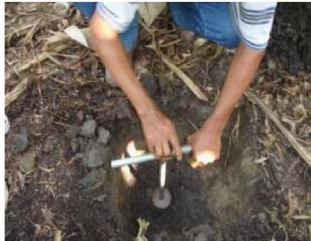
Figures 3 and 4. Sample extraction for soil analysis
