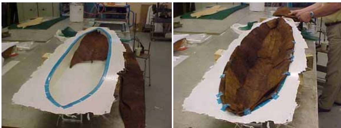
dry coir mats are placed into the mould
