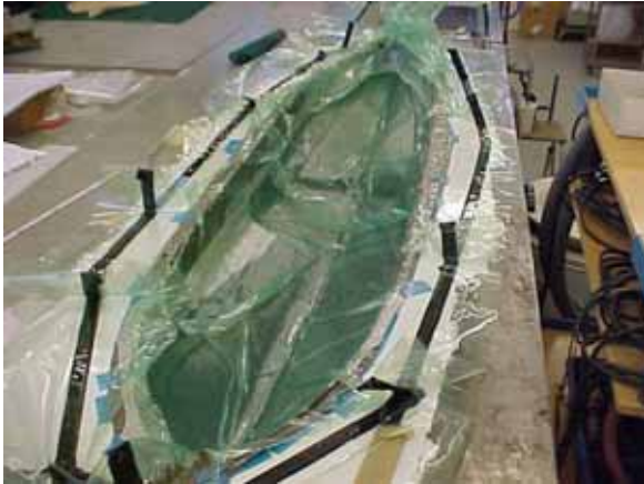
material is bagged, package is sucked vacuum and resin is let in
