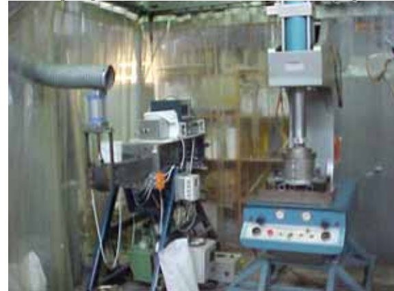
The setup with the extruder and 20 tons press
