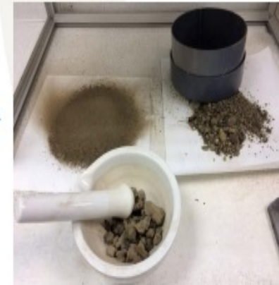
Disaggregation and sieving at 2 mm
