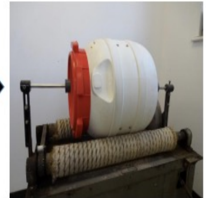
Homogenization with a barrel roller
