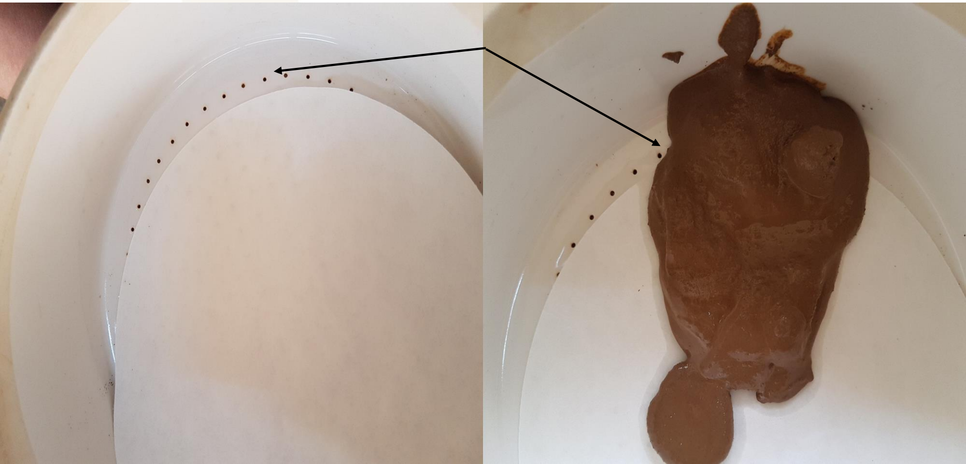
6- small size of filter paper or improperly placed
