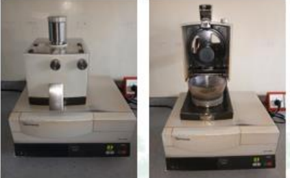
RM 200 Restch machine for grinding 2mm sieved soils to < 0.05 mm
