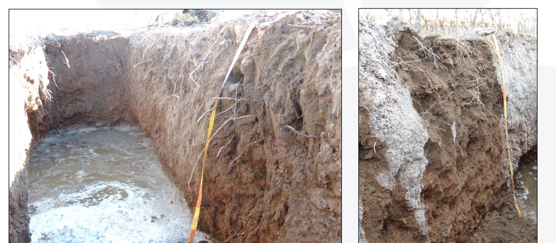
Figure 6. Also in the Lower Valley of the Neuquén River the influence of the water table in the low fluvial terrace accentuates the salinization process.
