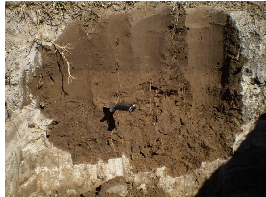
Salt deposits in surface from groundwater rises
