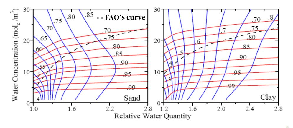
Iso-lines of relative transpiration,  $T_r = T_a/T_p$  (red) and relative mass leached below the root zone,  $L_r = M_L/M_T$  (blue);  $M_T = M_A + M_I$ ;  $Y_a/Y_p \approx T_a/T_p$ .
