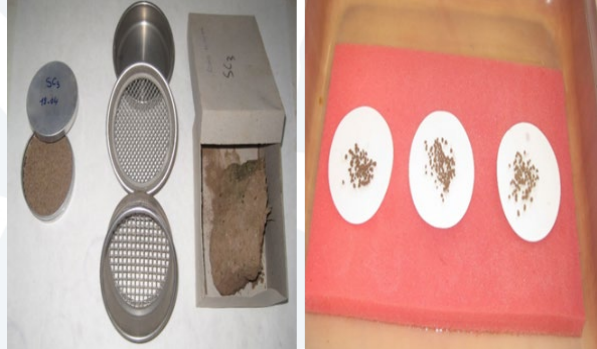
Structural stability Le Bissonais
