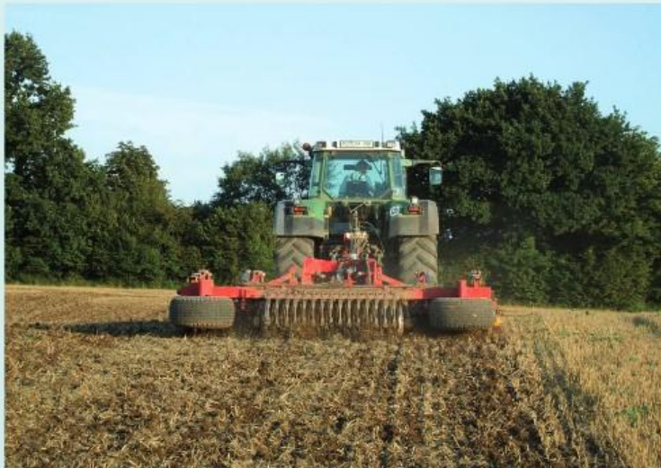
Disc harrow used for reduced tillage operations (Germany) (Source: Stephan Hubertus Gay)
