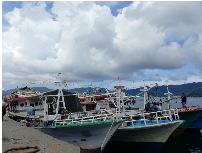
Fig.3. Small ring net “Pachekos” (5-20 GT) used to catch scads, small neritic tunas and skipjack in Bitung.
