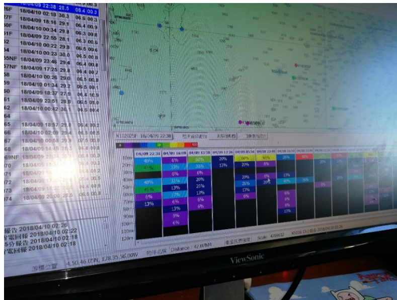
Fig. 3. Screen display of Kato echo-sounder buoys
