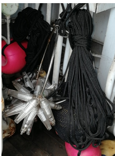
Fig. 1. Small cluster of LED lights used to hang under FAD before sets
