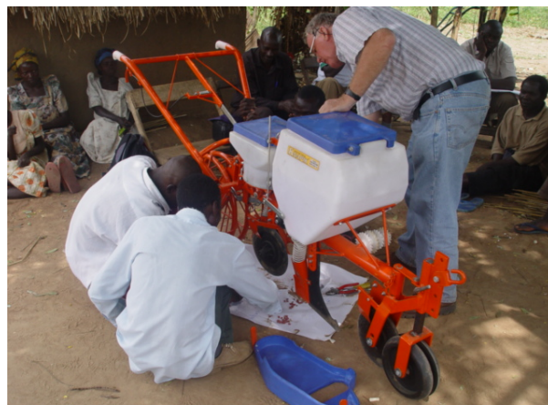
Fig. 2h: Demonstrating Calibration of a triton planter
