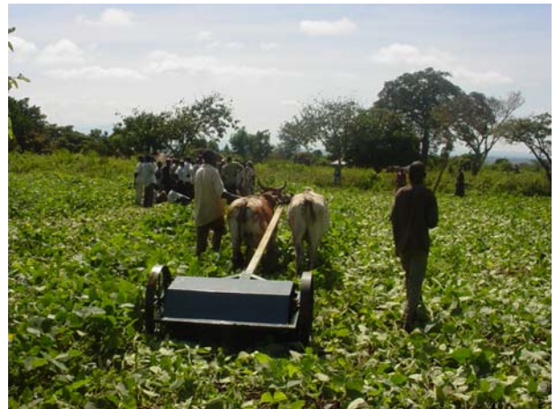
Fig. 2d: Soil cover (Mucuna) knocked down by an ox-drawn knife roller before direct planting
