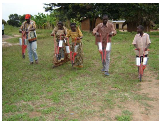
Fig. 2j : Farmers in Bulumbi FFS learning how to use a Jab planter
