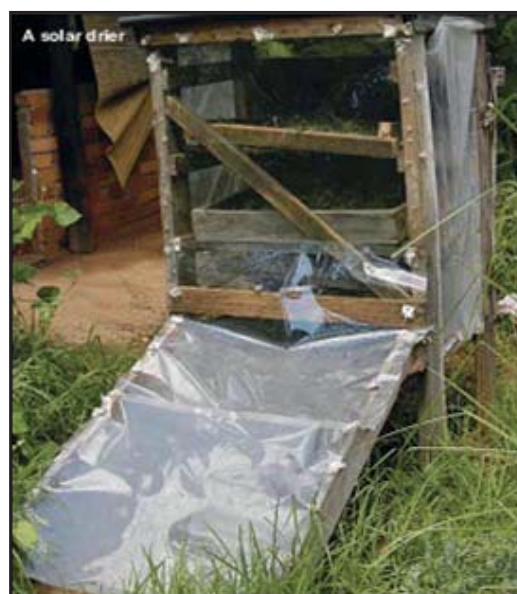
Pic. 20: A solar drier allows to dry foods on sun without exposing them to the direct sun light
