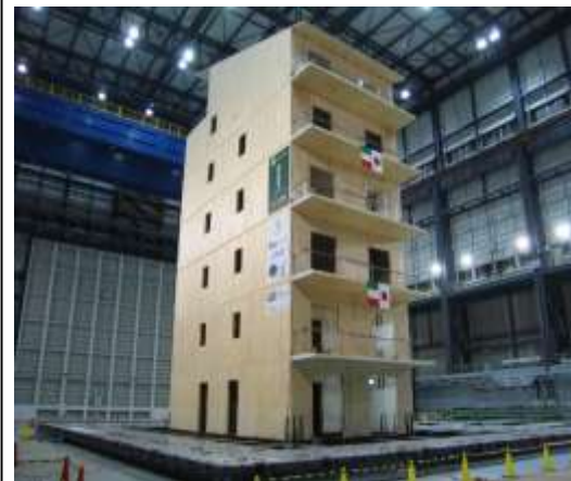
Earthquake test of 7 storey CLT building on earthquake shake table at Miki in Japan. Research collaboration between Ivalsa in Italy and Germany/Austria SOFIE Project
