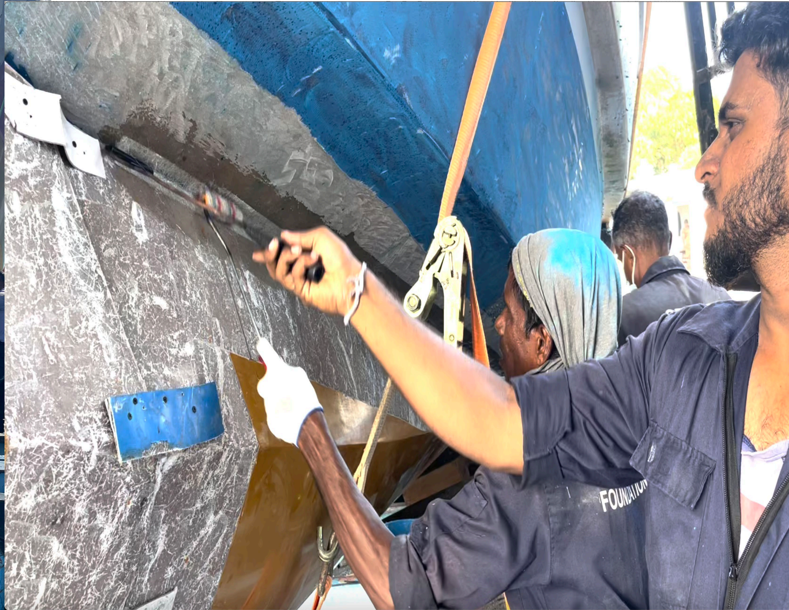
Fiberglassing the bulbous bow onto the hull.
