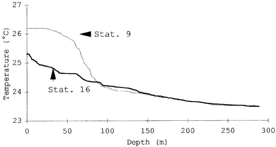
Figure 6. Two examples of Temperature depth profiles measured during this study by a CTD-12 probe. Note the difference in profiles in the upper 100m of depth between sampling station 16 (situated more South) and station 9 (North).
