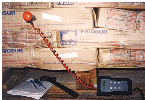
Figure 38.13: Measuring temperature within a carton.
