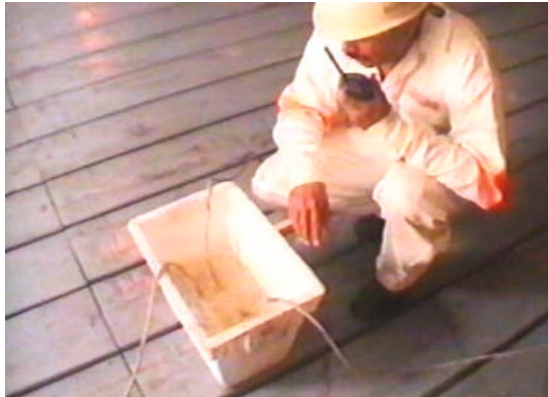
Figure 38.14: Reefer cargo temperature probe calibration.
