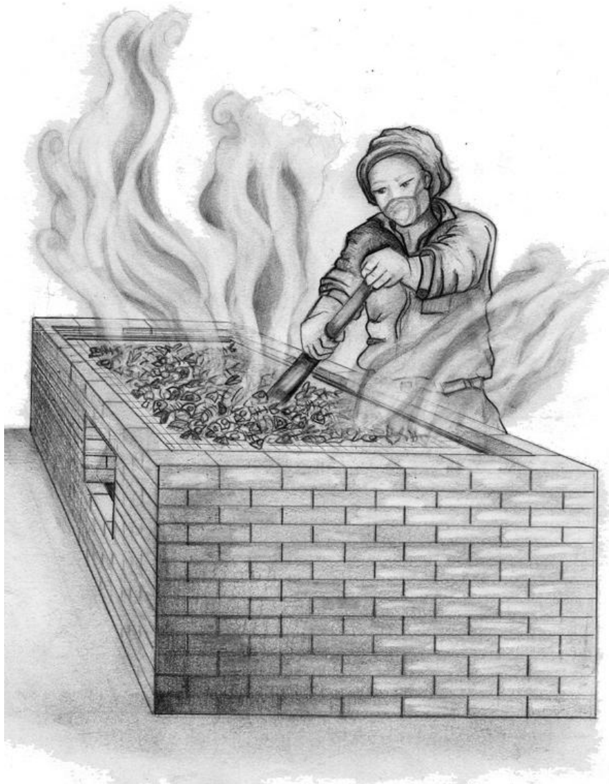
Figure 2: Class 2 animal feed is made by smoking and milling fresh fish remains.
