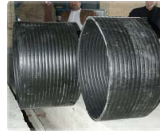
Poly-ethylene pipes for lining the qanat gallery
